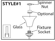
**STYLE#1** - Remove spinner nut from socket. Position glass on the fixture and secure with spinner nut. Install proper bulb type and wattage.
