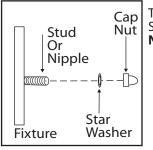
Tuck electrical wires into outlet box and position fixture over studs or nipple on mounting bracket assembly. Secure fixture in place with star washer(s) and cap nut(s). **Note:** If required, assemble body and spread the arms of the fixture out evenly.
